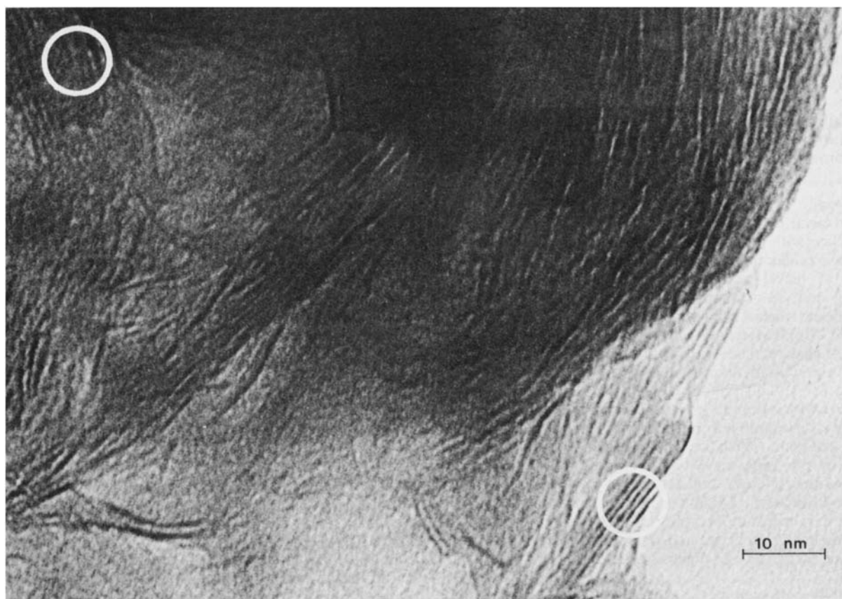
Figure 2. Transmission electron micrograph of Ni-SMM cross-linked with Si-Al oligomer.
